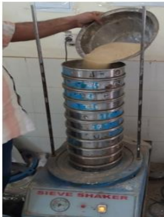
Fig 4: Sieve analysis test for coarse and fine aggregate were prepared to determine the tensile characteristics using an indirect tensile strength test. All tests were conducted following BS EN 206 [24]. The test results are summarized in Table 3.
