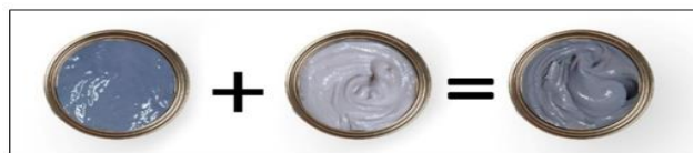
Fig 2: Mixing process of component B with component A, forming the resin matrix Sikadur®-330.
