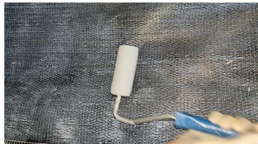
Fig 3: Impregnation by Sikadur®-330 as a resin using the manual hand layup method.
